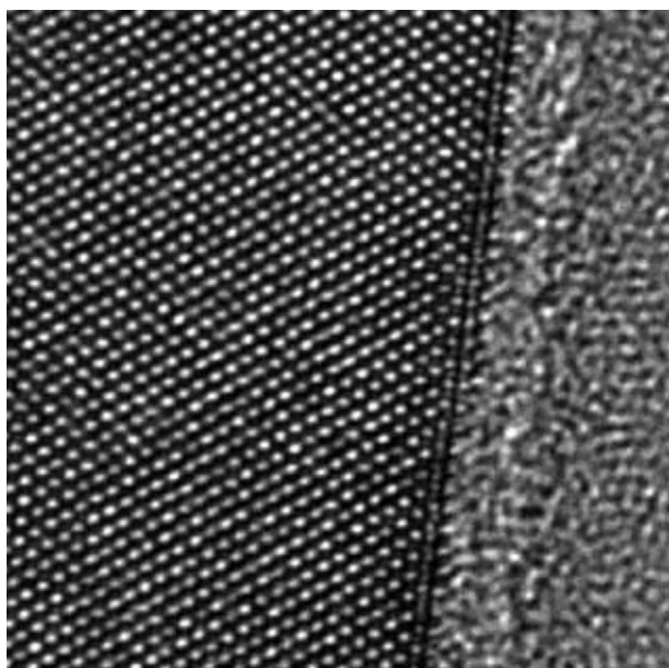
High-resolution bright field image of a Si/SiO x interface
